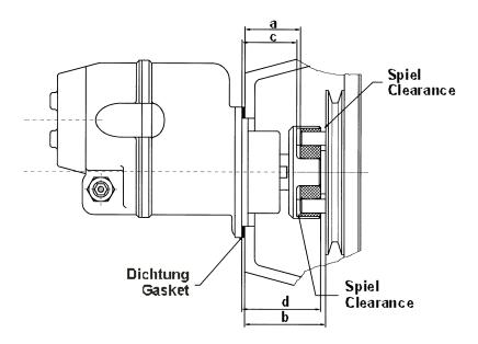
Caution: If there is any noticable resistance while turning the magneto before the locating pin is engaged, lift the pin slightly until the magneto drive can be turned. Do not force the magneto drive. After aprx. 10° rotation reinsert locating pin.
