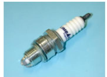
The electrode gap is not adjusted anymore on the new plugs. The factory adjustment may not be changed. Spark plug wear is not determined by erosion of the 3 ground electrodes. In use material is removed from the helper electrode (see bottom ill.). In extreme cases the helper electrode may be partially eroded.
