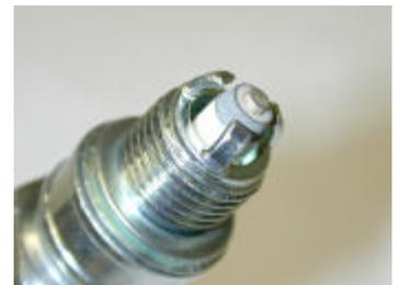
These spark plugs also require a special ignition harness as detailed in Technical Bulletin 63, because of the missing shielding.
