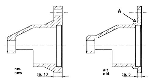
3. Replace old style starter shaft support with new unit P/No.: 202.143.201.000
