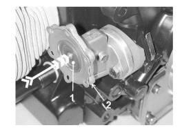
Remove o-ring and strainer from top of pump.
